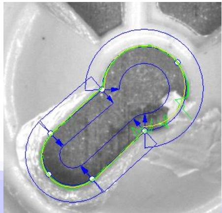
Many part inspection tasks work by comparing the part under scrutiny to a reference shape. Deviations from it form protrusions or intrusions which you want to detect.
