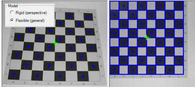
An image is said to be calibrated when a mapping has been established between the pixel coordinates and some real-world coordinate system established on the observed surface.
