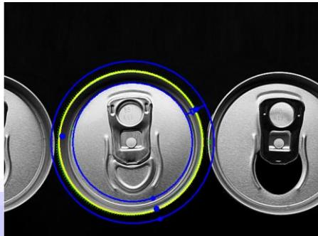
Gauging enables very accurate measurements of edges in order to determine positions, distances, sizes, angles...
